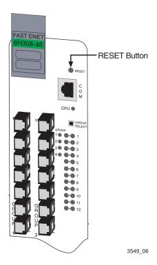
To reset the module processor, press and release the RESET button. The module goes through a reset process for approximately 60 seconds. Additional downtime may result as the module reenters the network.
